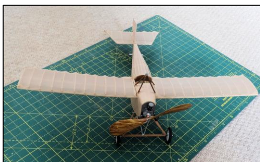
1911 Caudron N peanut - Just waiting to add rigging wires. Bare airframe only weighed 6 grams but with covering, engine, prop and wheels it's now about 13 grams! At least it is very slightly nose heavy.
